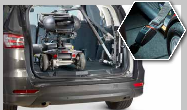
4 The seatbelt restraint ensures your mini scooter or wheelchair is safely stowed
